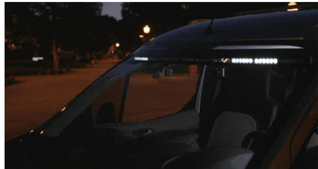
Fig. 7: Ford has proposed a light bar on the windshield to communicate the intent of the vehicle [14].
