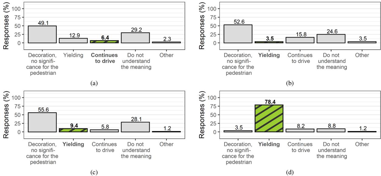
Fig. 8: Distribution of how the vehicle's intent was interpreted when the vehicle was approaching the pedestrian. The intention of the vehicle is highlighted in green. (a) Ford's LED light strip signaling it is continuing to drive; (b) Ford's LED light strip signaling it is stopping to yield; (c) Mercedes-Benz' LED panel signaling it is stopping to yield; (d) Mercedes-Benz projecting on the road it is stopping to yield.
