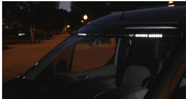
Fig. 7: Ford has proposed a light bar on the windshield to communicate the intent of the vehicle [14].
